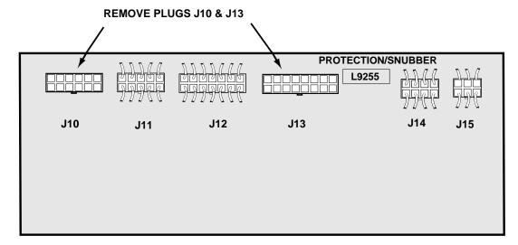
FIGURE F.13 - PROTECTION/SNUBBER BOARD PLUG LOCATIONS.
